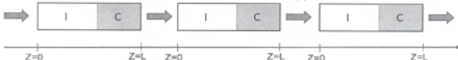
Fig. 2. Axial coordinate values in a succession of the inert and catalyst zones for a three bed network (I - inert; C- Catalyst)
